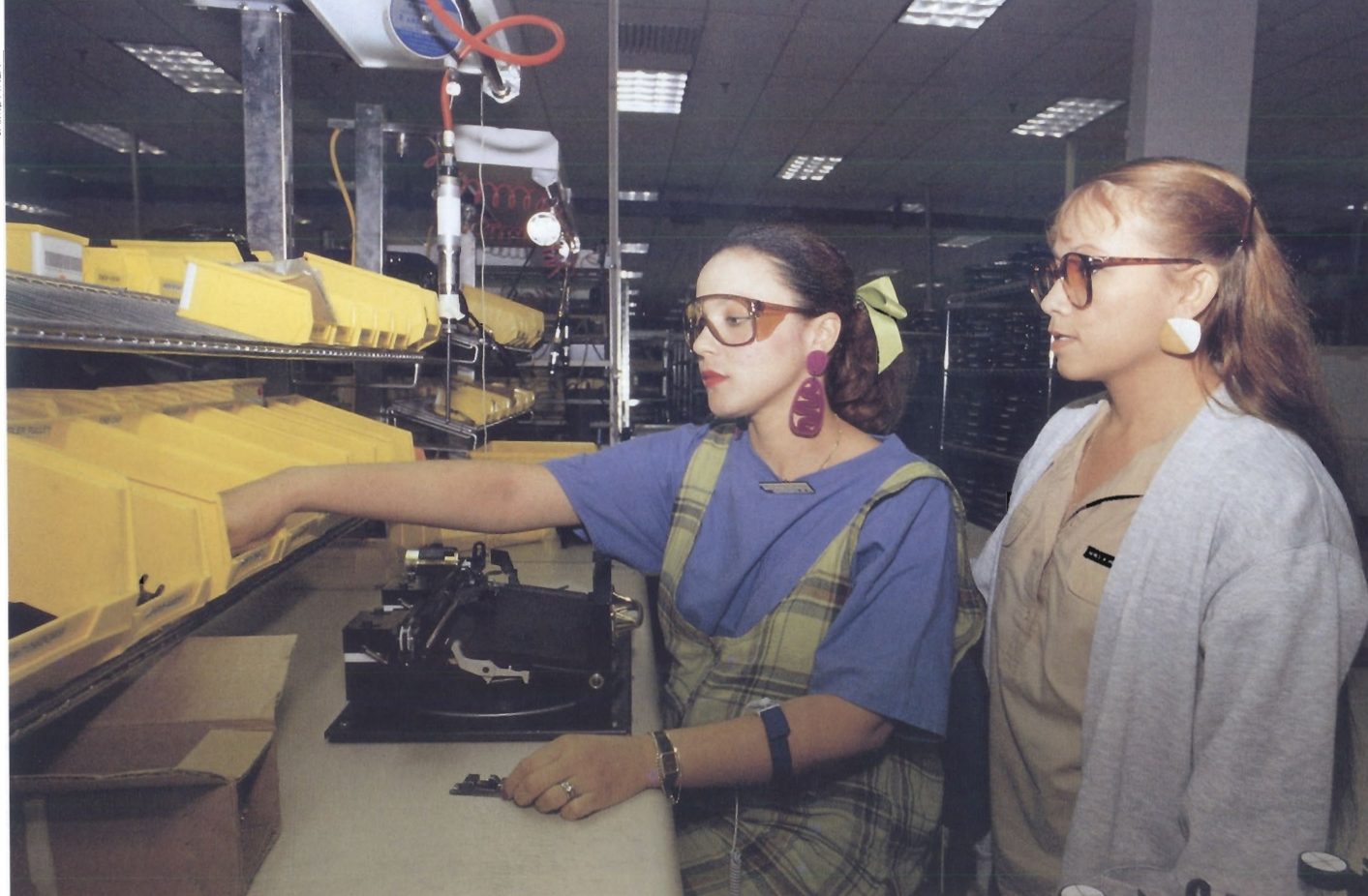
Blanca Rivera (left) confers with Marta Perez while hand loading components on a chassis. PRMO began building computer video-display terminals in 1980 and now manufactures more than 60 networking and memory products.
