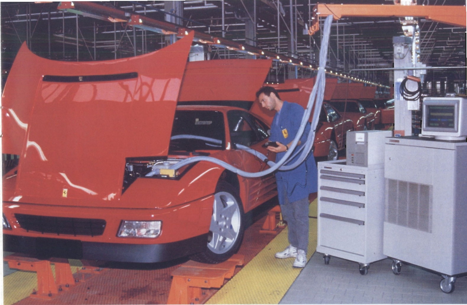
Equipment from HP's Advanced Manufacturing Systems Operation tests the electrical system of the Ferrari 348 at four of the 20 work sites.
